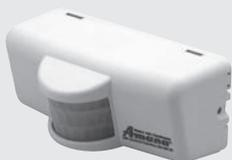
The **DigiSmart Occupancy Sensor and Door Switch Combo Device** completes the in-room equipment. This infrared sensor can determine whether the room is occupied or empty and when empty, signal the PTAC to adjust the temperature to save energy based on programmable set-backs.
