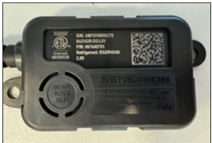
FIGURE 23. Example of Clear, Unobstructed Sensor Inlet
