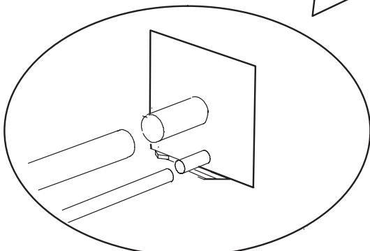
**F PLACE A WET RAG AGAINST PIPING PLATE AND AROUND THE SUCTION LINE CONNECTION.**
