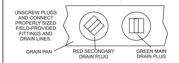
**FIGURE 14. Drain Line Connections**
