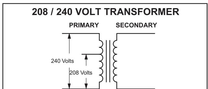
**FIGURE 20. Converting Unit from 240VAC to 208VAC**
