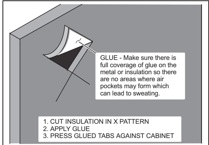
**FIGURE 21. Repairing Insulation**
