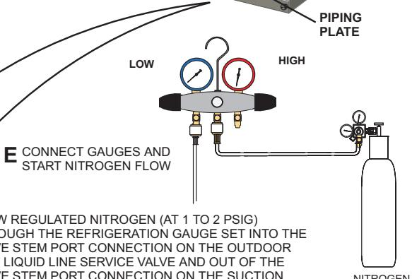
FLOW REGULATED NITROGEN (AT 1 TO 2 PSIG) THROUGH THE REFRIGERATION GAUGE SET INTO THE VALVE STEM PORT CONNECTION ON THE OUTDOOR UNIT LIQUID LINE SERVICE VALVE AND OUT OF THE VALVE STEM PORT CONNECTION ON THE SUCTION SERVICE VALVE.
