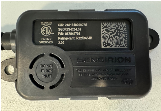
FIGURE 7. Example of Clear, Unobstructed Sensor Inlet
