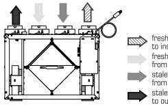
fresh air to inside fresh air from outside stale air from inside stale air to outside
