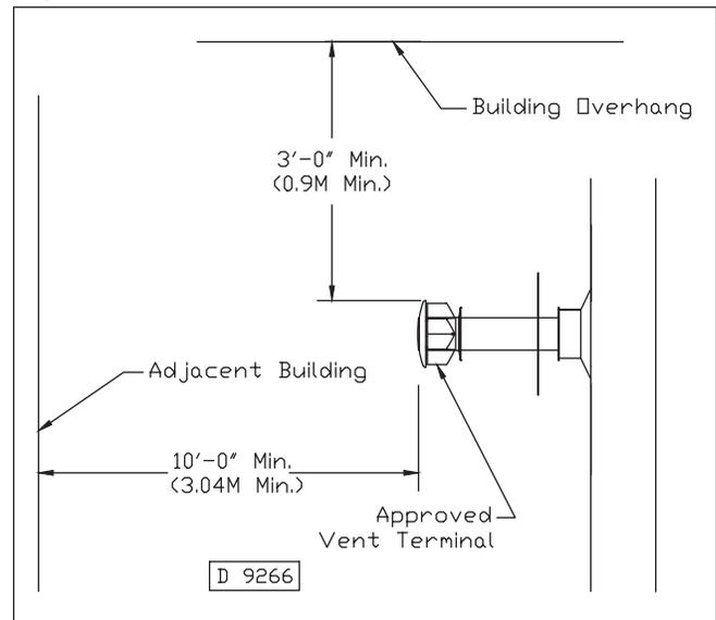
**Figure 5 - Horizontal Vent Termination**
