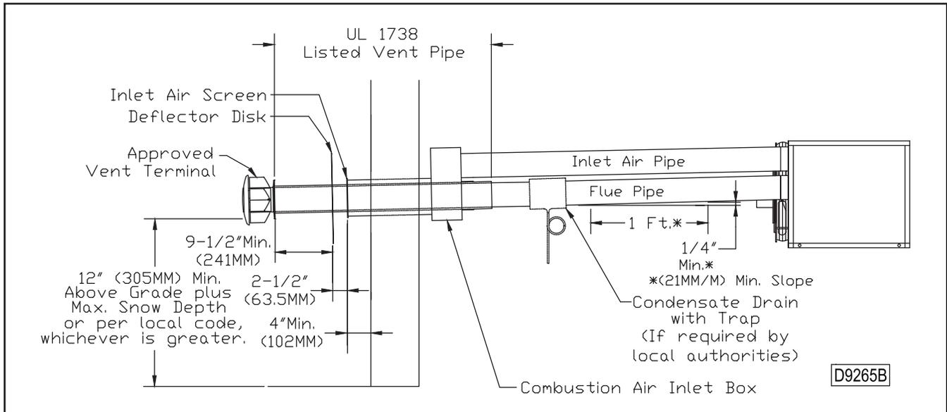
**▲ WARNING** Never use pipe other than 4 inch diameter. Never use PVC, ABS or any other nonmetallic pipe for venting! To do so may result in serious damage to the unit and or severe personal injury or death!
