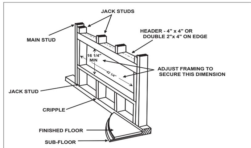
Wall sleeve opening height should be squared with wall sleeve opening width.
