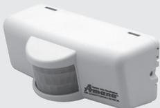
The **DigiSmart Occupancy Sensor and Door Switch Combo Device** completes the in-room equipment. This infrared sensor can determine whether the room is occupied or empty and when empty, signal the PTAC to adjust the temperature to save energy based on programmable set-backs.
