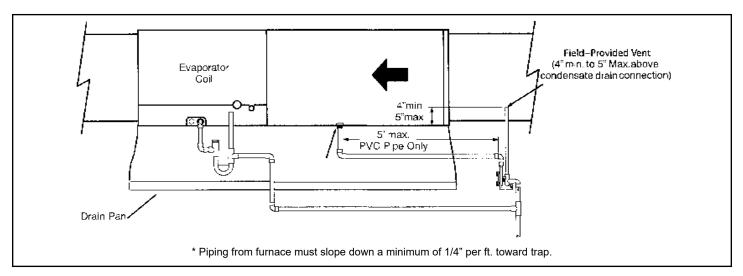
Figure 57. Evaporator Coil Using a Common Drain (Unit shown in horizontal left-hand discharge position)
