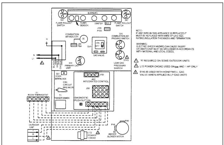
Figure 66. Typical Field Wiring Diagram
