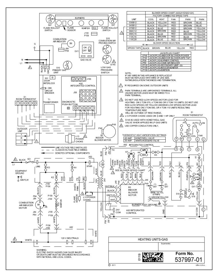
Figure 67. Typical Wiring Diagram
