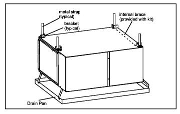
Figure 19. Typical Horizontal Application
