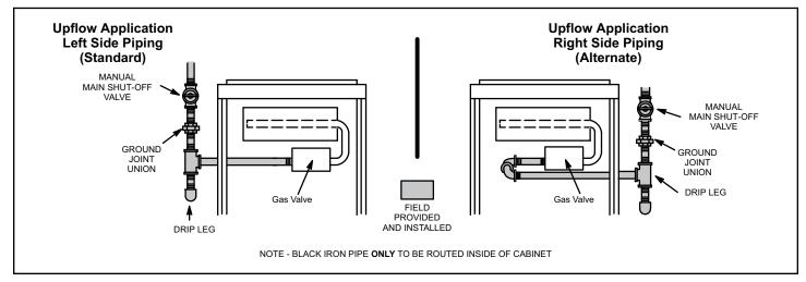
Figure 61. Gas Piping Upflow Applications
