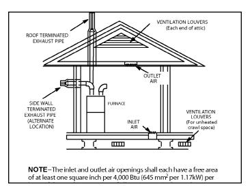
Figure 6. Equipment in Confined Space - All Air from
