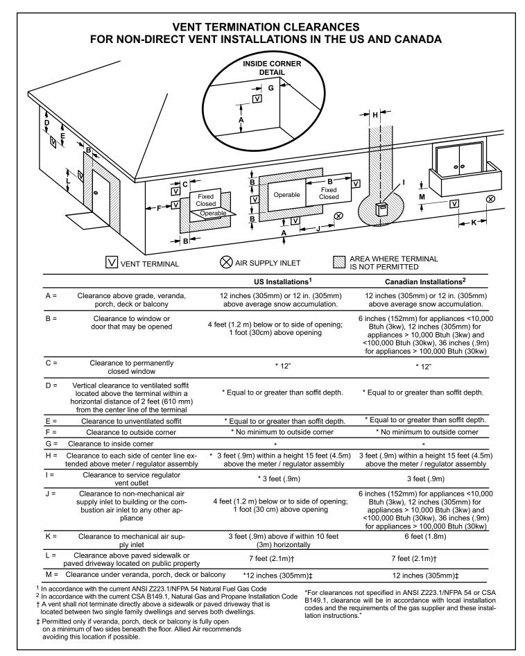
Figure 34. Vent Termination Clearances for Non-Direct Vent Installations
