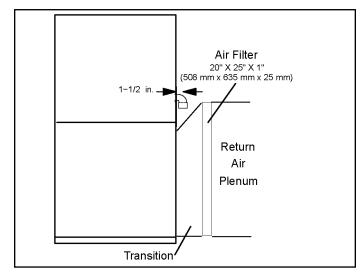
Figure 14. Side Return Air (with Transition and Filter)
