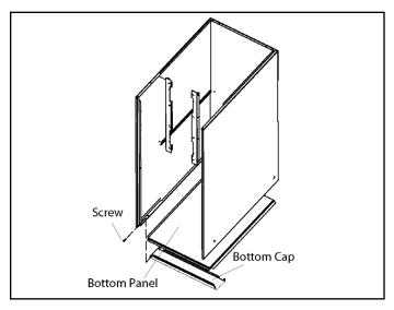
Figure 16. Removing the Bottom Panel
