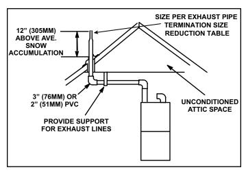
Figure 45. Non-Direct Vent Roof Termination Kit (15F75 or 44J41)
