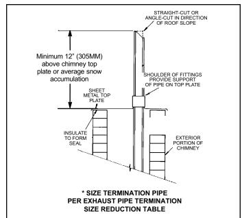
**NOTE**: Do not discharge exhaust gases directly into any chimney or vent stack. If vertical discharge through an existing unused chimney or stack is required, insert piping inside chimney until the pipe open end is above top of chimney and terminate as illustrated. In any exterior portion of chimney, the exhaust vent must be insulated.
