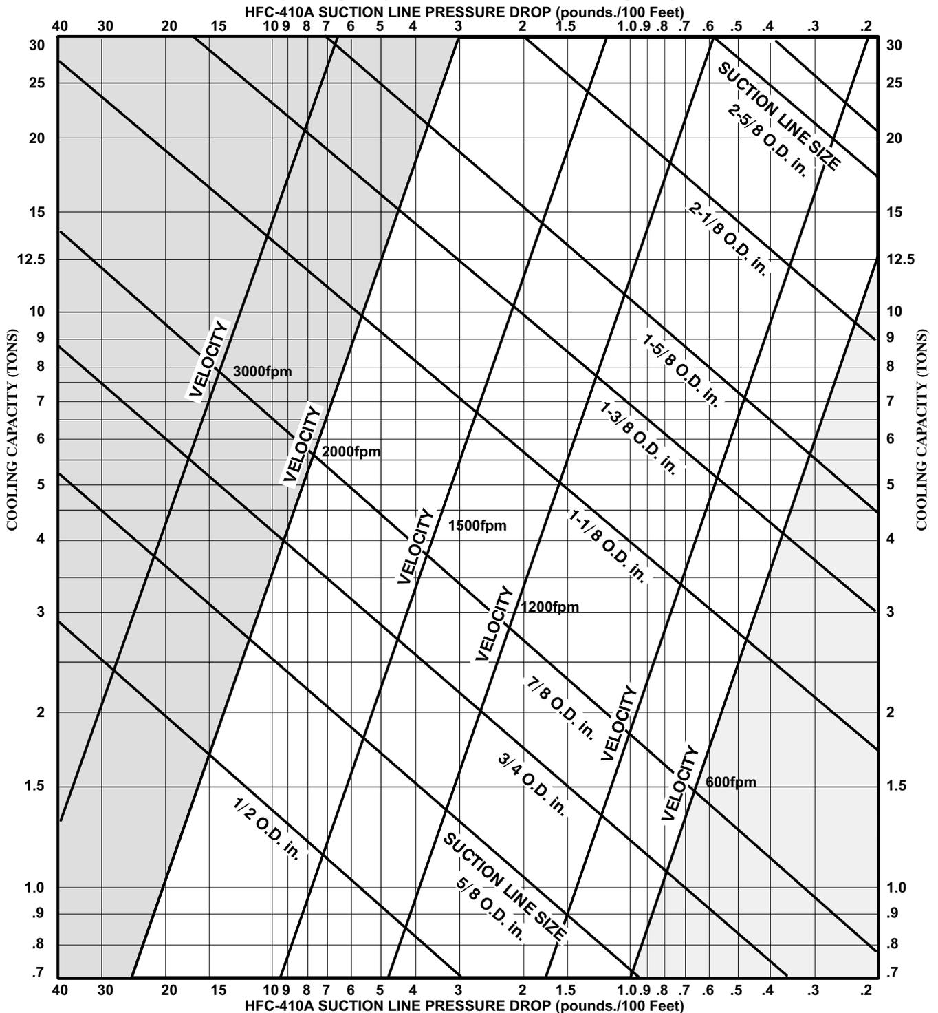
To use this chart, first find capacity (tons) on left side of chart. To find pipe size, proceed right to smallest pipe size. Pressure drop (vertical line) and velocity (diagonal lines) can then be determined for the pipe size selected. For example, for 10 ton unit, select 1-3/8 in. outside diameter. line.
