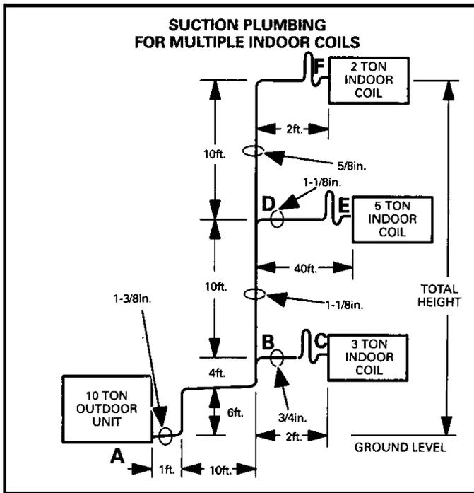
**Figure 24. Suction Plumbing for Multiple Indoor Coils**
