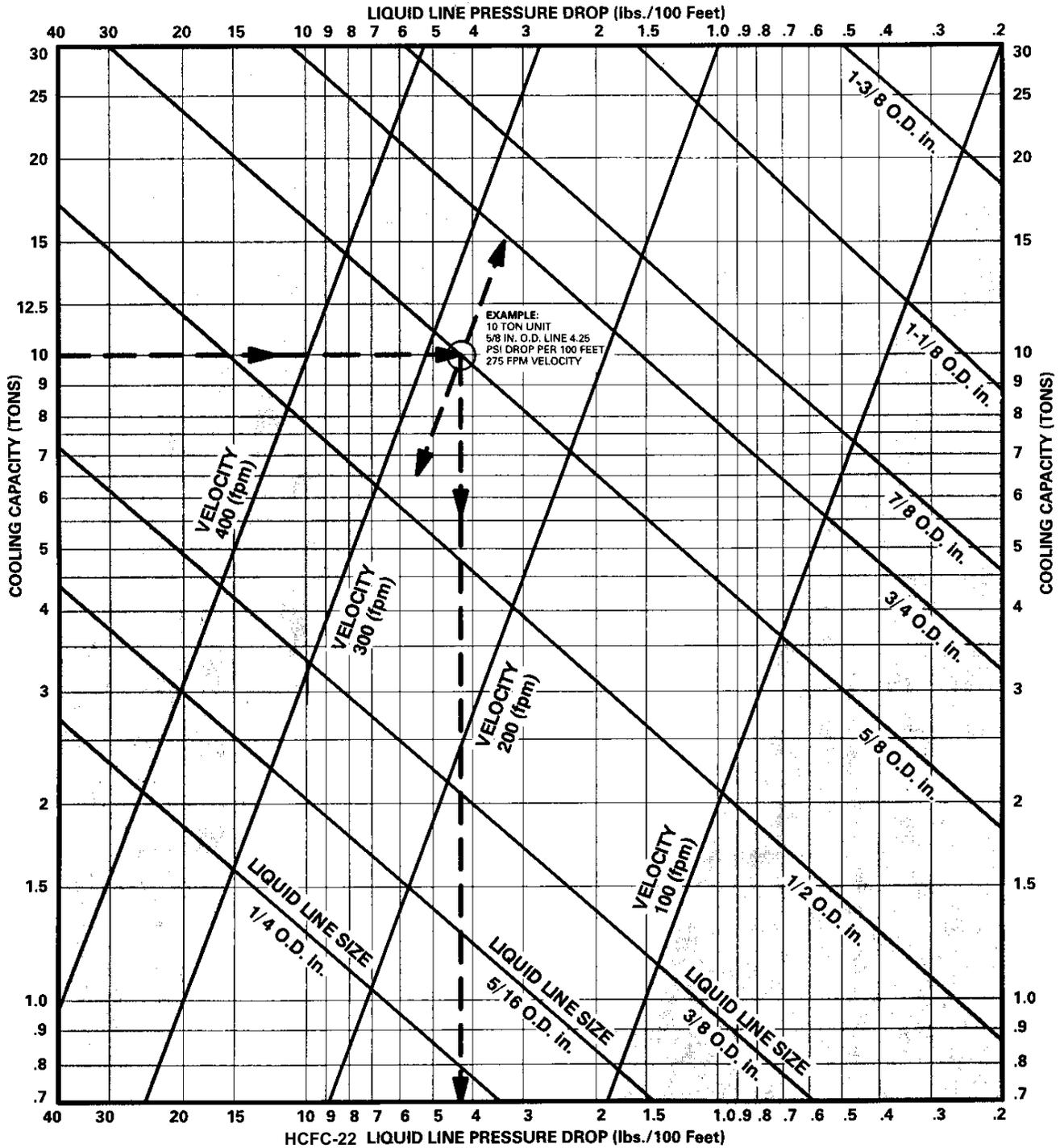
To use this chart, first find capacity (tons) on left side of chart. To find pipe size, proceed right to smallest pipe size. Pressure drop (vertical line) and velocity (diagonal lines) can then be determined for the pipe size selected. For example, for 10 ton unit, select 5/8 in. O.D. line.
