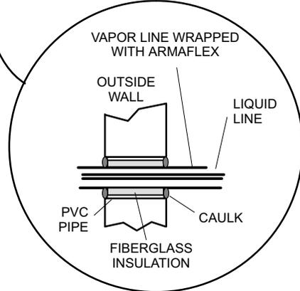
**NOTE** — Similar installation practices should be used if line set is to be installed on exterior of outside wall.
