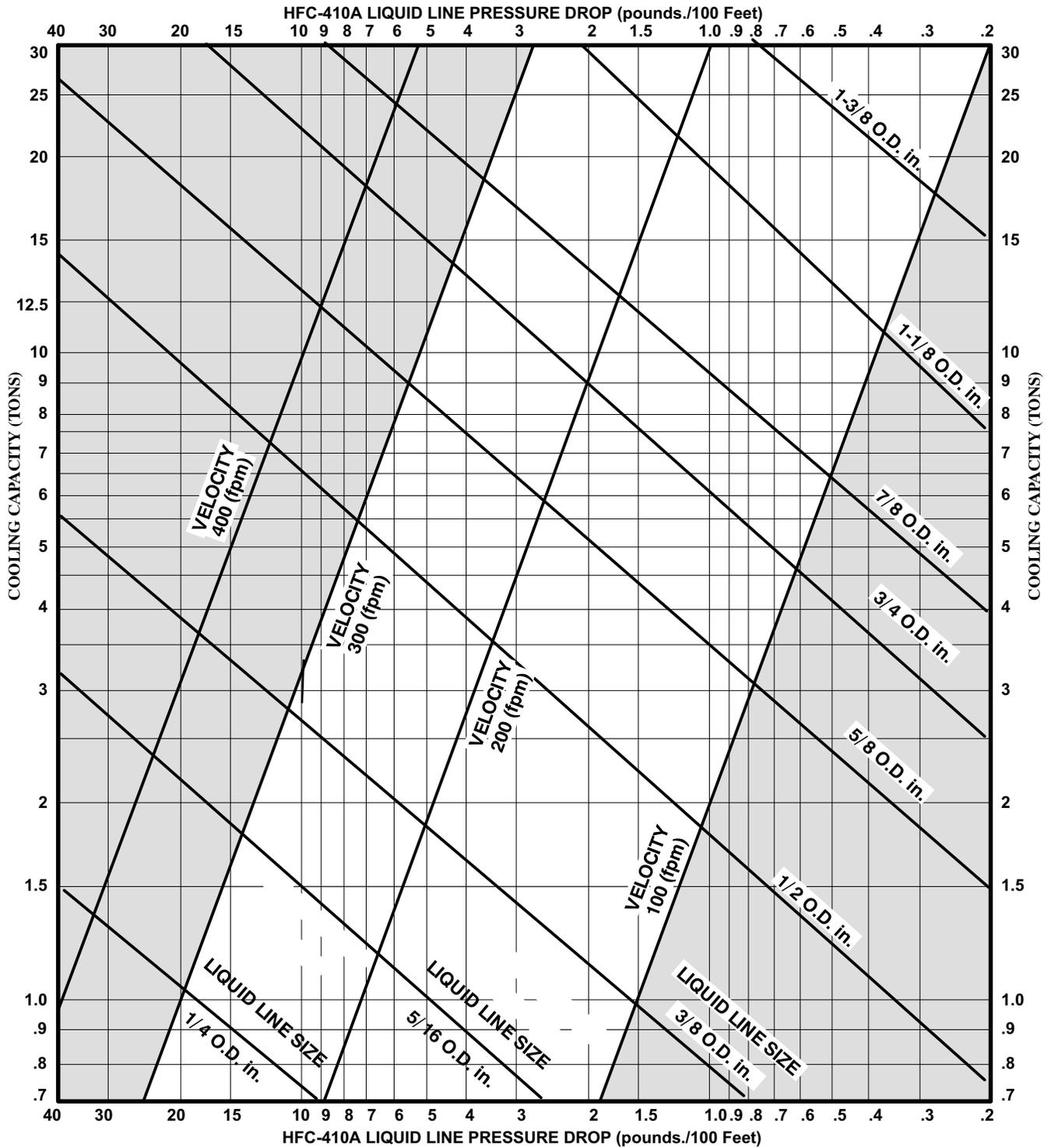
To use this chart, first find capacity (tons) on left side of chart. To find pipe size, proceed right to smallest pipe size. Pressure drop (vertical line) and velocity (diagonal lines) can then be determined for the pipe size selected. For example, for 10 ton unit, select 5/8 in. outside diameter. line.
