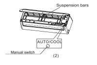
**NOTE:** The unit must be turned off before operating the manual control button. If the unit is operational, continue pressing the manual control button until the unit is off. ① Open and lift the front panel up to an angle
