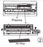
Hold the two parts of Plasma where are marked with  $\clubsuit$  signal and lift it. Then you can open the cover of the the plasma and remove the filter.
