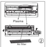
Hold the two parts of Plasma where are marked with  $\uparrow$  signal and lift it. Then you can open the cover of the the plasma and remove the filter.
