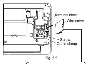
The Wiring Diagram is located on the inside of the indoor unit's wire cover.
