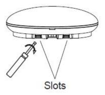
• Now insert the WFCC WiFi module into the receptacle under the lid as shown. You should feel it click securely into place.
