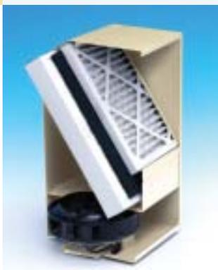
**Unit features three filters positioned for added efficiency.** Prefilter and carbon filter should be changed every three months. HEPA filter is designed to last from two to five years depending on the the level of pollutants in your home.
