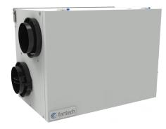
Fantech's, SER 200 is an Energy Recovery Ventilator designed for higher static pressure applications. The unit brings a continuous supply of fresh air into a home while exhausting an equal amount of contaminated air. The energy recovery core at the center of the unit transfers heat and moisture from incoming air to the outgoing air that was cooled and dried by the building's air conditioner.
