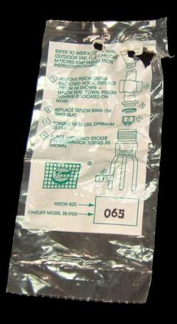
4. Remove bag contents: orifice, O-ring, and wire.
