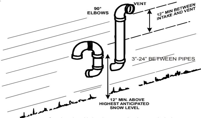
Combustion Air Intake may also be snorkeled to obtain 12" min ground clearance.
