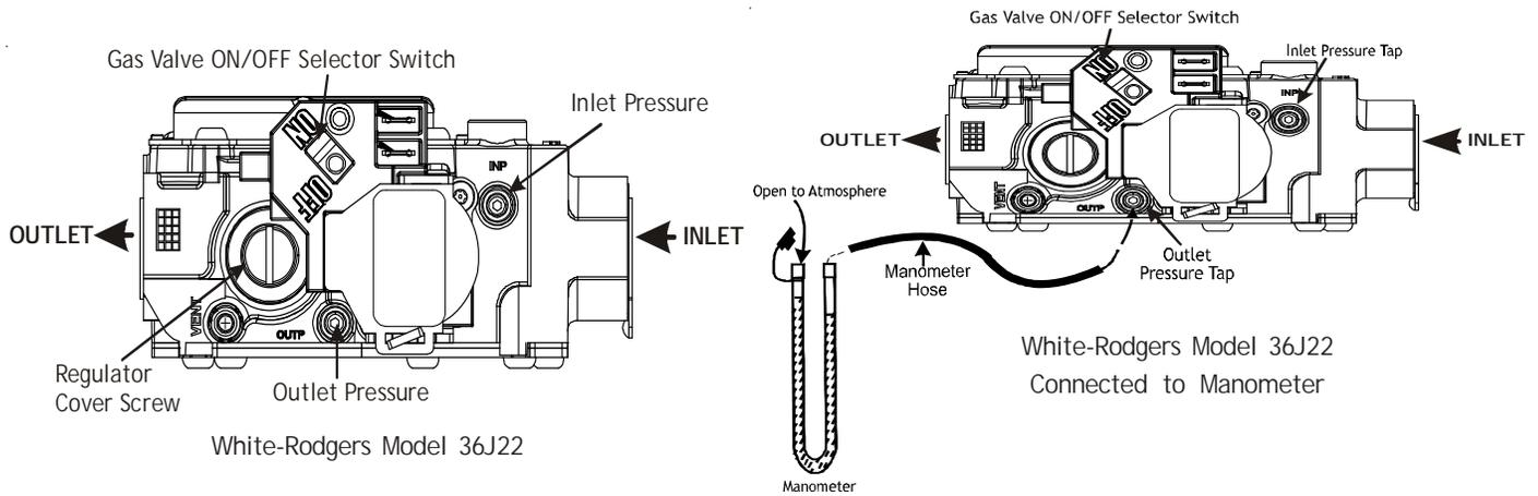
If supply pressure differs from table, make the necessary adjustments to pressure regulator, gas piping size, etc., and/or consult with local gas utility.
