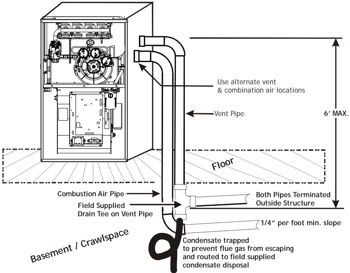
*All piping and fittings must be joined per material manufacturer's specifications to prevent separation and flue gas leaks.*
