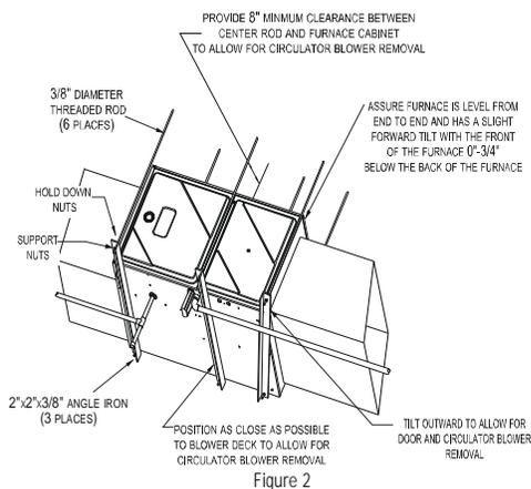
When installing a furnace horizontally, additional consideration must be given to the following:
