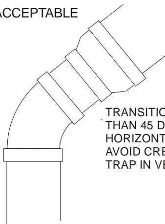
TRANSITION NO LESS THAN 45 DEGREES TO HORIZONTAL PLANE TO AVOID CREATING A WATER TRAP IN VENT PIPING.
