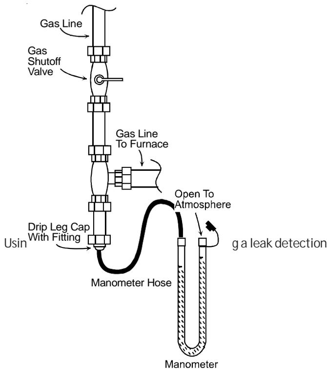
Measuring Inlet Gas Pressure (Alt. Method)
