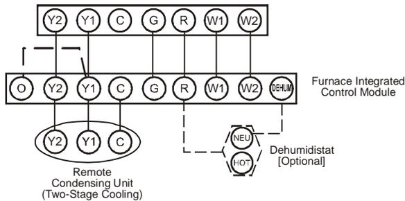
Thermostat - Two-Stage Heating with Two-Stage Cooling
