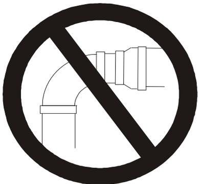
NO TRANSITION ON HORIZONTAL PLANE, THIS CREATES A WATER TRAP AND RESTRICTS FLUE GASES
