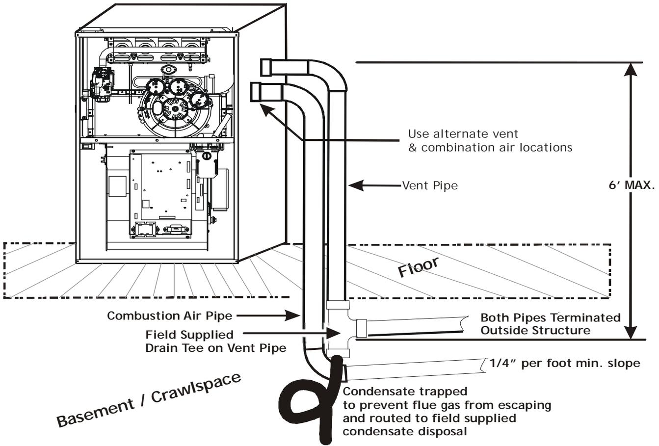
*All piping and fittings must be joined per material manufacturer's specifications to prevent separation and flue gas leaks.*
