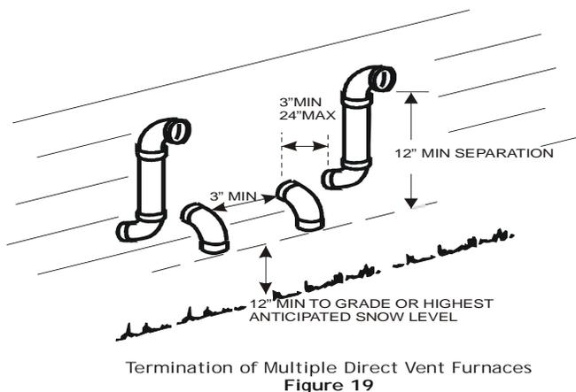
The vent/flue and combustion air pipes may terminate vertically, as through a roof, or horizontally, as through an outside wall.
