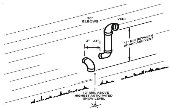
Alternate Horizontal Vent Termination (Dual Pipe)
