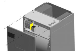
Install the four SPW-01 kit wires to the circuit breaker lugs and torque lug screws to 35 in-lbs. Ensure all wires are tucked inside the control box.
