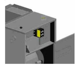
Install the four SPW-01 kit wires to the circuit breaker lugs and torque lug screws to 35 in-lbs. Ensure all wires are tucked inside the control box.
