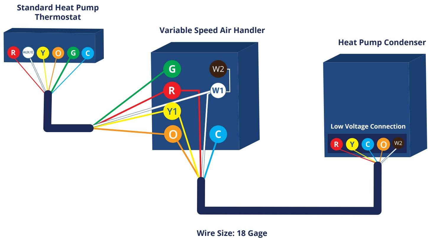
This diagram is to be used as reference for the low voltage control wiring of your heating and AC system. Always refer to your thermostat or equipment installation guides to verify proper wiring.
