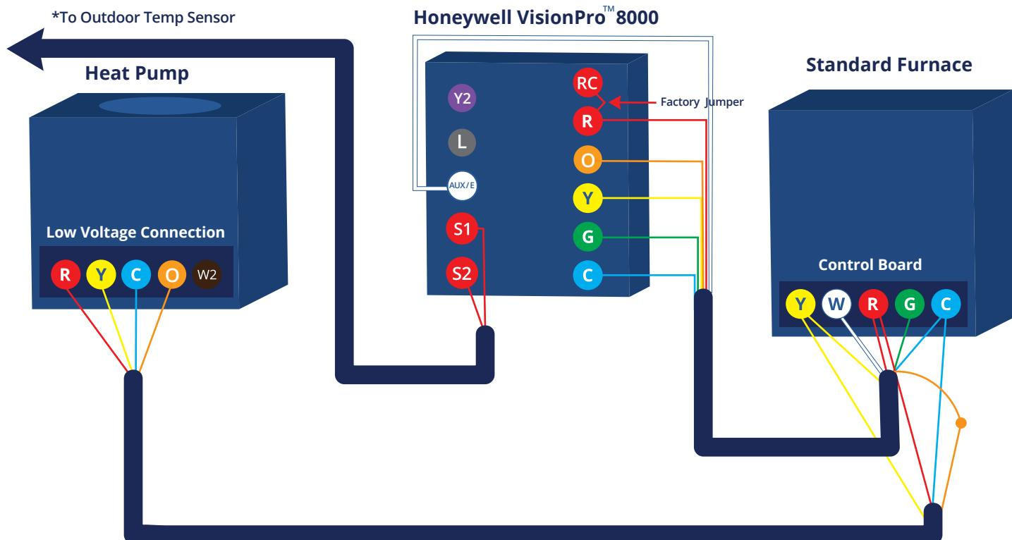
This diagram is to be used as reference for the low voltage control wiring of your heating and AC system. Always refer to your thermostat or equipment installation guides to verify proper wiring.
