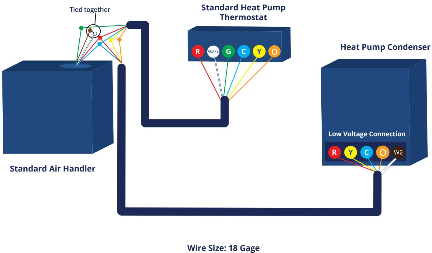
This diagram is to be used as reference for the low voltage control wiring of your heating and AC system. Always refer to your thermostat or equipment installation guides to verify proper wiring.
