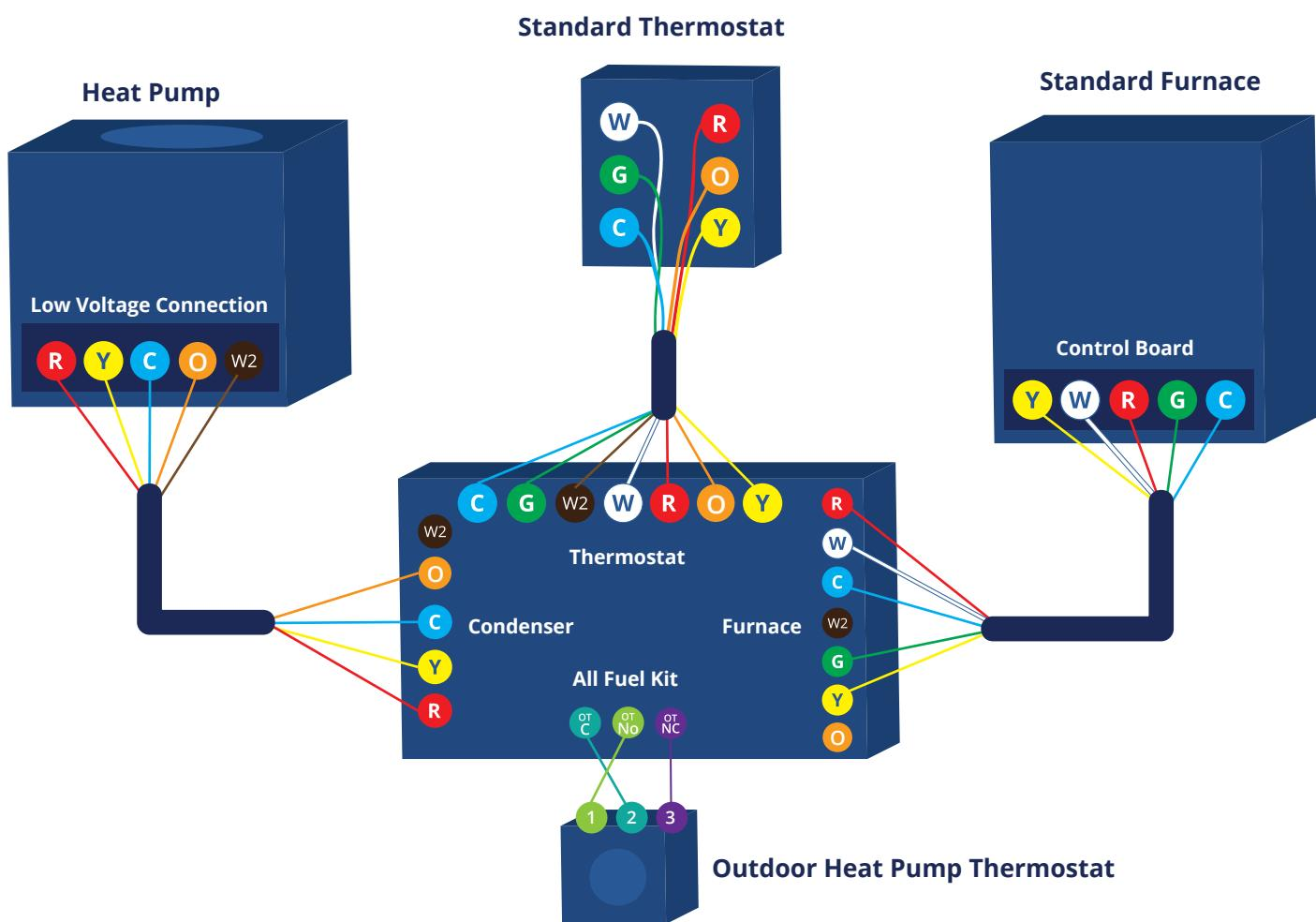
This diagram is to be used as reference for the low voltage control wiring of your heating and AC system. Always refer to your thermostat or equipment installation guides to verify proper wiring.
