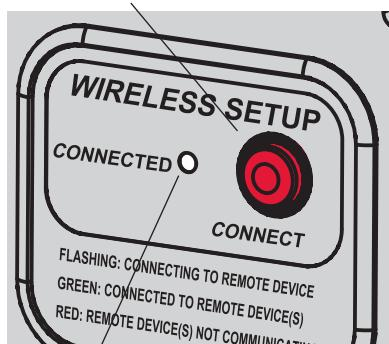
Press the **CONNECT** button at the EIM or wireless adapter and wait for green flashing light to begin linking devices to the wireless network (see page 3).
