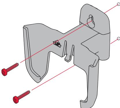
Mount the sensor on a vertical exterior wall, at least 6 inches below any overhang. Choose a location protected from direct sunlight.
