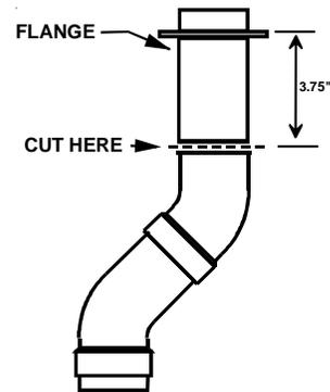
Vent/Flue Pipe Cuts
