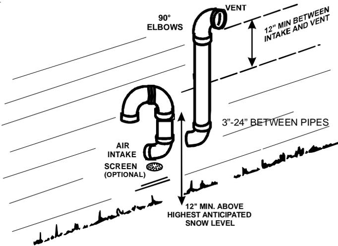
Combustion Air Intake may also be snorkeled to obtain 12" min ground clearance.
