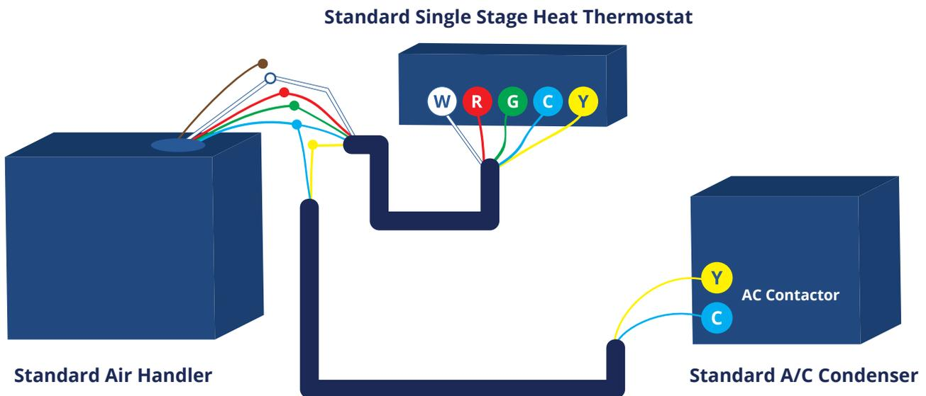
This diagram is to be used as reference for the low voltage control wiring of your heating and AC system. Always refer to your thermostat or equipment installation guides to verify proper wiring.
