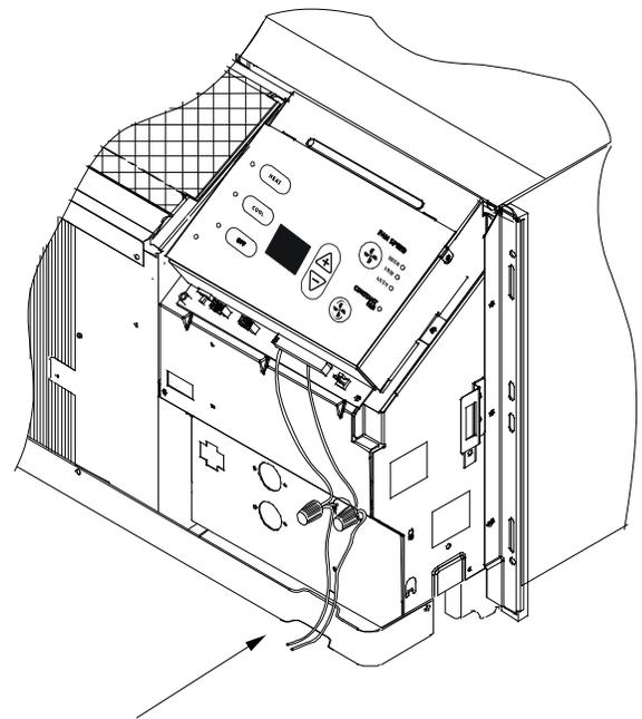
No holes are permitted in chassis basepan or wallsleeve when routing low voltage wire. Route the low voltage wires through the indentation on the front of the basepan.
