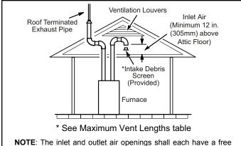
**NOTE**: The inlet and outlet air openings shall each have a free area of at least one square inch per 4,000 Btu (645 mm<sup>2</sup> per 1.17 kW) per hour of the total input rating of all equipment in the enclosure.
