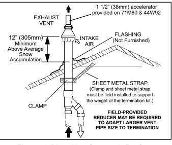
Figure 40. Direct Vent Concentric Rooftop Termination 71M80, 69M29 or 60L46 (US) 44W92 or 44W93 (Canada)
