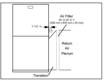
Figure 14. Side Return Air (with Transition and Filter)
