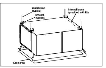
Figure 19. Typical Horizontal Application
