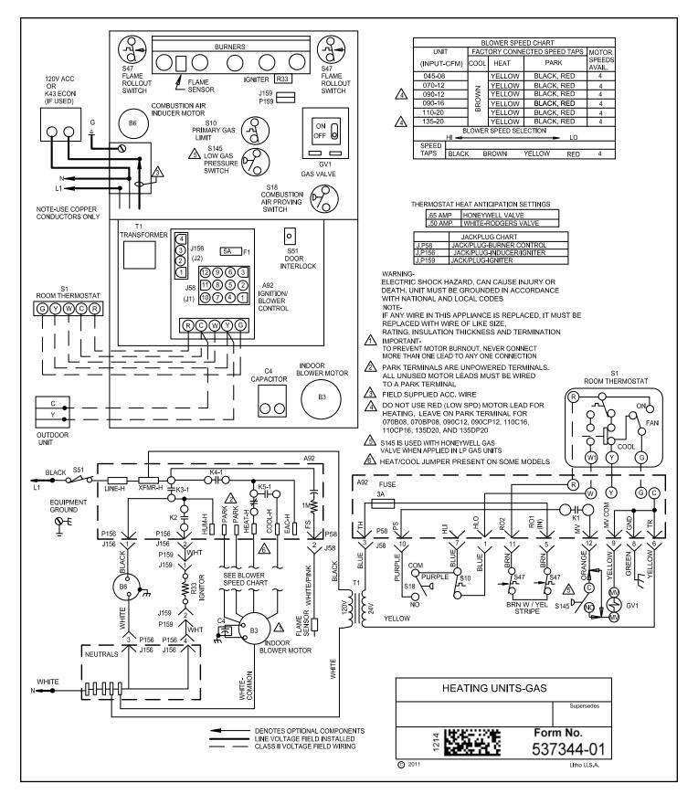
Figure 67. Typical Wiring Diagram
