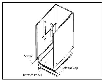
Figure 16. Removing the Bottom Panel
