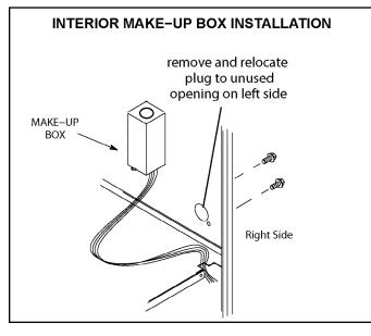
The unit is equipped with a field makeup box. The makeup box may be moved to the right side of the furnace to facilitate installation. Seal unused openings on left side with plugs removed from right side. Secure the excess wire to the existing harness to protect it from damage.
