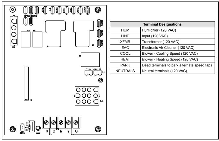
Figure 68. Integrated Control (Automatic Hot Surface Ignition System)
