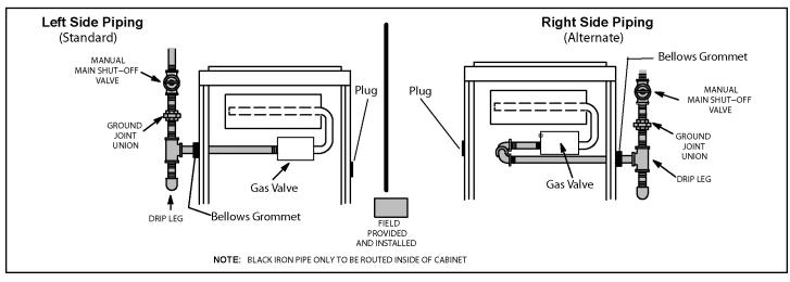
Figure 61. Gas Piping Upflow Applications
