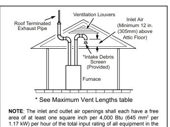
enclosure. Figure 31. Equipment in Confined Space
