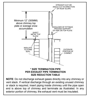
Figure 48. Non-Direct Vent Application Using Existing Chimney
