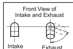
**1** The exhaust termination tee should be connected to the 2" or 3" PVC flue pipe as shown in the illustration. Do not use an accelerator in applications that include an exhaust termination tee. The accelerator is not required.
