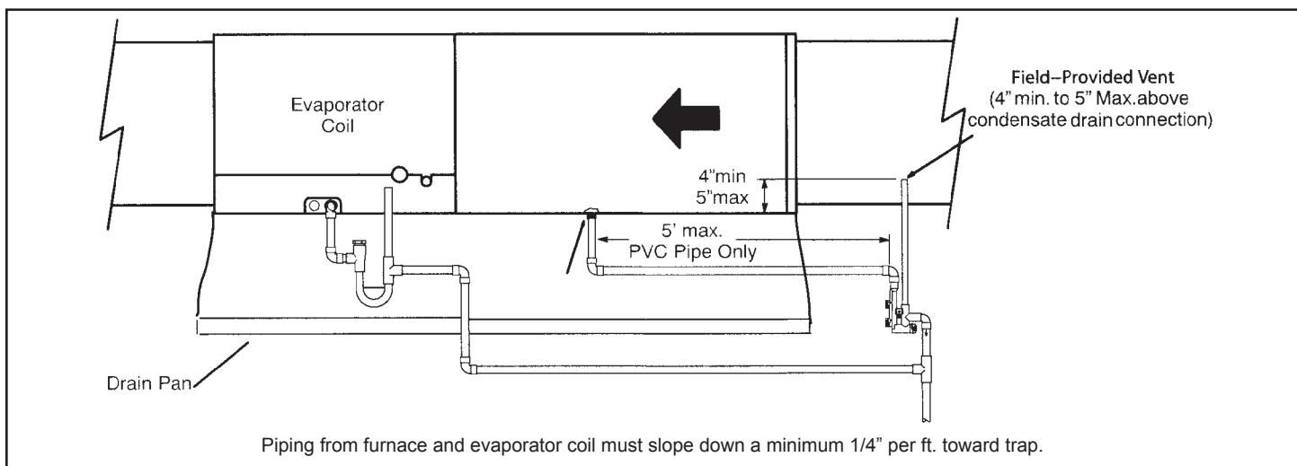
Figure 58. Evaporator Coil Using a Common Drain
