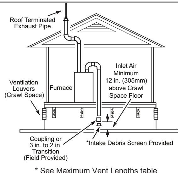
**NOTE:** The inlet and outlet air openings shall each have a free area of at least one square inch per 4,000 Btu (645mm<sup>2</sup> per 1.17kW) per hour of the total input of all equipment in the enclosure.
