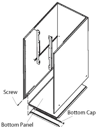
**Figure 16. Removing the Bottom Panel**
