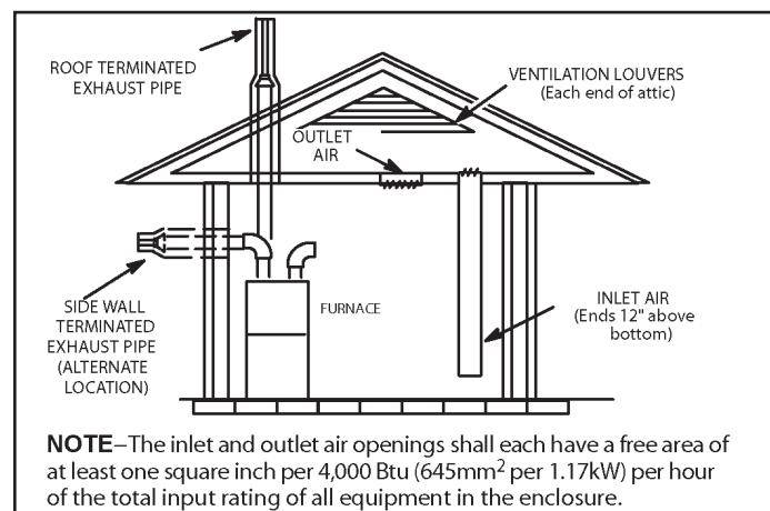
**NOTE** – The inlet and outlet air openings shall each have a free area of at least one square inch per 4,000 Btu ( $645 \text{ mm}^2$  per 1.17kW) per hour of the total input rating of all equipment in the enclosure.
