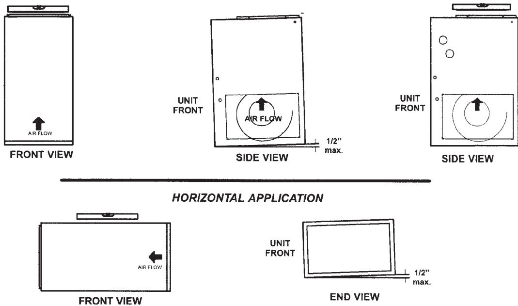
Tilt the unit slightly (Max. 1/2") from back to front to aid in the draining of the heat exchanger.
