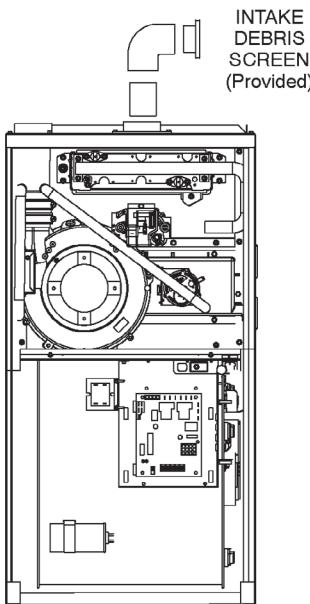
**NOTE** – Debris screen and elbow may be rotated, so that screen may be positioned to face forward or to either side.
