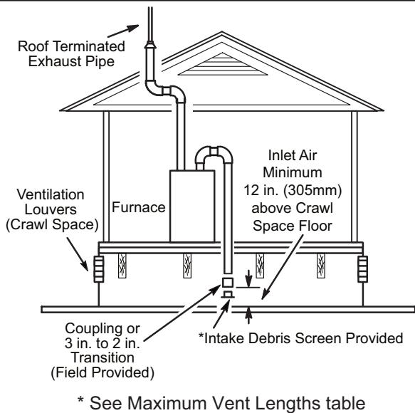
**NOTE:** The inlet and outlet air openings shall each have a free area of at least one square inch per 4,000 Btu (645mm<sup>2</sup> per 1.17kW) per hour of the total input of all equipment in the enclosure.
