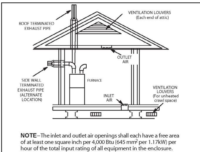
**NOTE** – The inlet and outlet air openings shall each have a free area of at least one square inch per 4,000 Btu ( $645 \text{ mm}^2$  per 1.17kW) per hour of the total input rating of all equipment in the enclosure.
