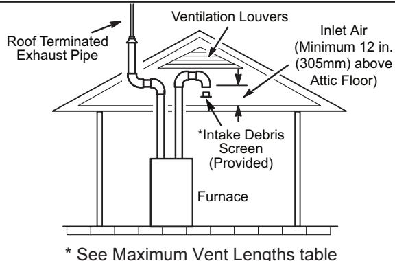
**NOTE:** The inlet and outlet air openings shall each have a free area of at least one square inch per 4,000 Btu (645mm<sup>2</sup> per 1.17kW) per hour of the total input of all equipment in the enclosure.
