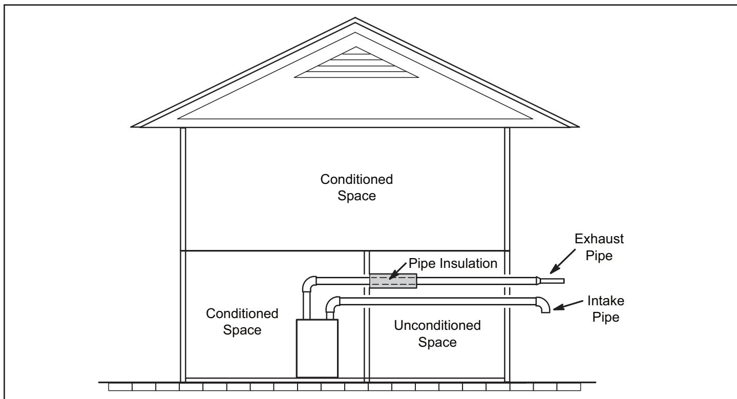
**Figure 33. Insulating Exhaust Pipe in an Unconditioned Space**
