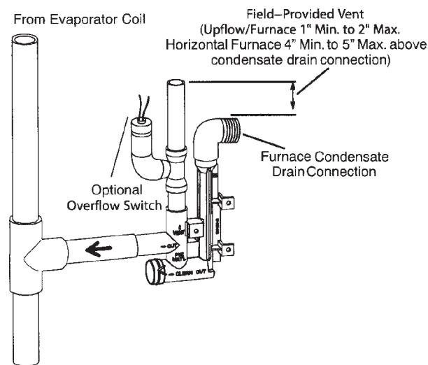
**Figure 54. Condensate Trap with Optional Overflow Switch**
