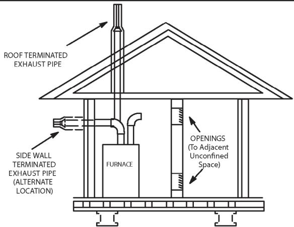
**NOTE** – Each opening shall have a free area of at least one square inch per 1,000 Btu ( $645 \text{ mm}^2$  per .29kW) per hour of the total input rating of all equipment in the enclosure, but not less than 100 square inches ( $64516 \text{ mm}^2$ ).
