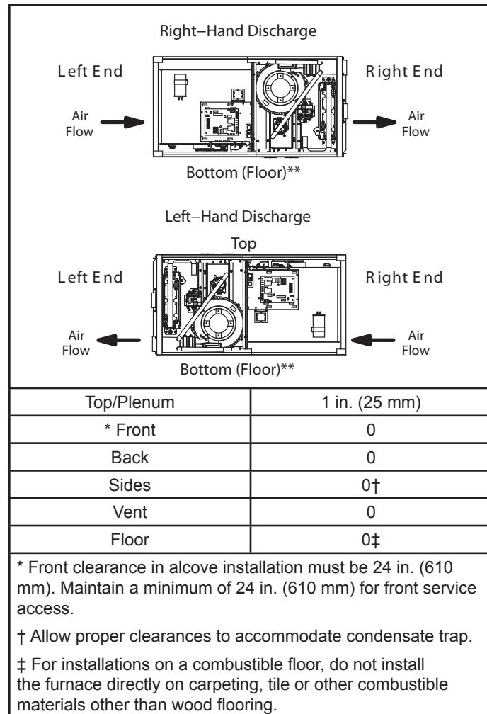
**Figure 18. Installation Clearances
