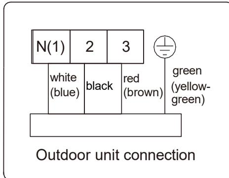
(5). Electric wiring of indoor unit side
