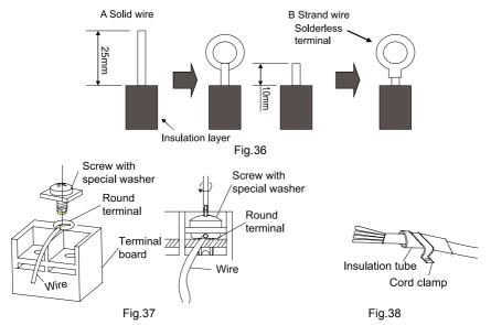
(3). How to fix connection cord and power cord by cord clamp
