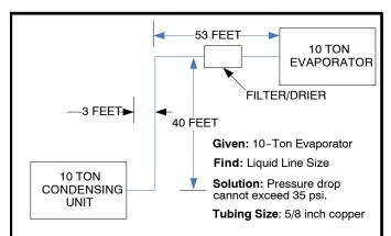
Two  $90^{\circ}$  long radius elbows @ 5/8 inch O.D. = 1 foot equivalent feet each.
