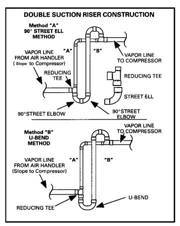
Figure 17. Double Suction Riser Construction
