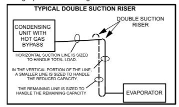
Figure 14. Typical Double Suction Riser
