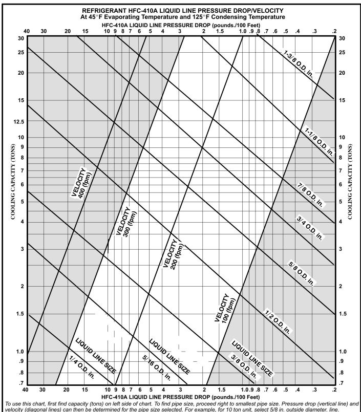
velocity (diagonal lines) can then be determined for the pipe size selected. For example, for 10 ton unit, select 5/8 in. outside diameter. line.
