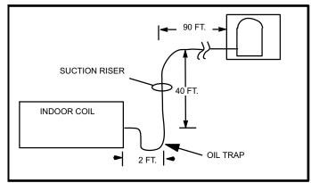
Figure 2. Indoor Coil Below Condenser
