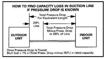
Figure 10. How to Find Capacity Loss
