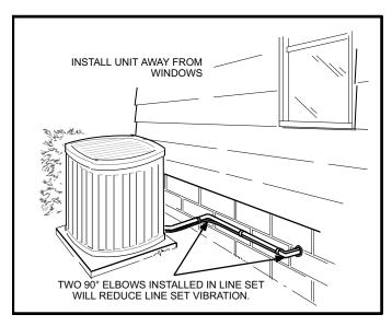
Figure 21. Outside Unit Placement
