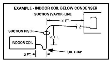
Figure 12. Indoor Coil Below Condenser
