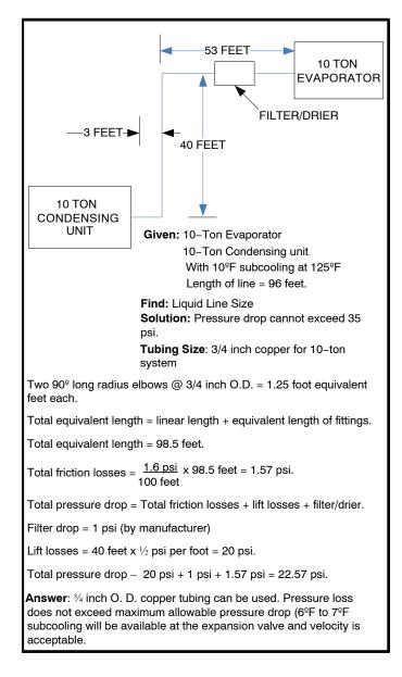
Figure 9. Liquid Line Sizing Example (Alternative)
