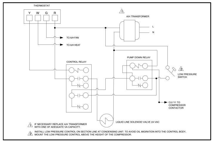
Figure 19. Non-Recycling Pump Down Control - Field Wiring Diagram
