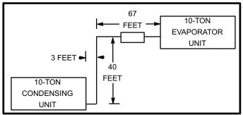
Figure 1. Liquid Line Sizing Example
