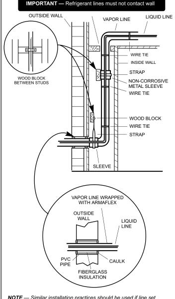
**NOTE** — Similar installation practices should be used if line set is to be installed on exterior of outside wall.
