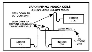
Figure 23. Vapor Piping Indoor Coils above and below Main
