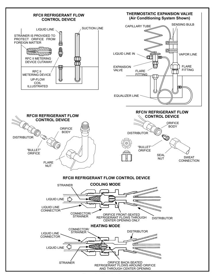
Figure 25. Metering Devices
