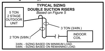
Figure 15. Typical Sizing - Double Suction Riser
