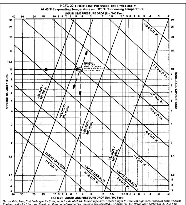
line) and velocity (diagonal lines) can then be determined for the pipe size selected. For example, for 10 ton unit, select 5/8 in. O.D. line. NOTE-Shaded area denotes unacceptable velocity range.
