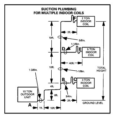
Figure 24. Suction Plumbing for Multiple Indoor Coils Find: Select tube size from figure 6.
