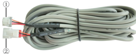
Fig. 23: Schematic diagram of connection wire: Connect terminal① with wired controller CN1; connect terminal ② with the terminal ④ of patch cord
