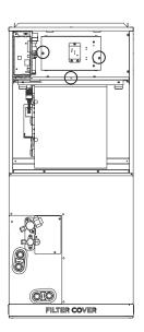
3. Install the electric auxiliary heating assembly into the chassis shell from the front, and note that the front end needs to be inserted into the shell assembly hole.
