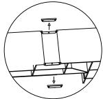
Remove knockouts as shown in the figure.
