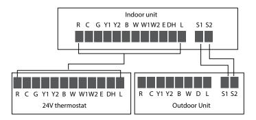
When using a 24v thermostat, please refer to the noncommunicating wiring diagrams that follow: (For this method you can use a thermostat with C wire connection for power. Wifi and higher end thermostats require C wire connections. Only one fan speed can be connected)
