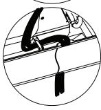
Replace foam gasket over wires.
