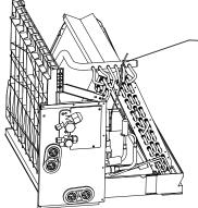
Use cable ties to fix the room temperature sensor as shown in the figure.
