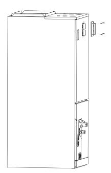
9. After installing the electric auxiliary heat module, apply the circuit breaker label near the silicone breaker cover that was just applied.
