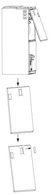
2. Remove the terminal block and power wires, loosen the screws, and remove the electric auxiliary heating cover.
