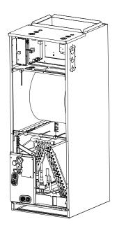
8. Reinstall the evaporator and drain pan.
