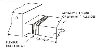
The outlet side pipe length is 1.5m/59".
