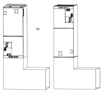
**Fixing instructions:** When installed vertically (upward or downward), the lower end of the air outlet needs to be connected to the L-shaped metal air duct and fastened by screws.
