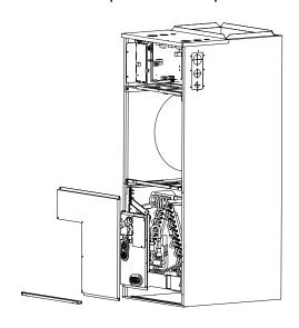
4. Unplug temperature sensors T1, T2, T2A, T2B and electronic expansion valve (EEV) from the control board.
