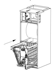
9. Reinstall T1, T2, T2A, T2B sensor plug, and electronic expansion valve (EEV) and tie up the sensor wires.
