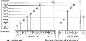
S4-1 DIP switch off Perform disconnection and short-circuit to achieve partition, control or dehumidification
