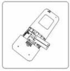
Remove batteries from remote control
