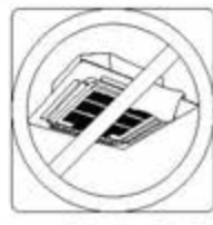
Make sure nothing is blocking all air inlets and outlets
