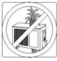
Make sure nothing is blocking all air inlets and outlets
