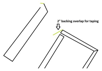
Step 3: Use foil tape to close up the plenum. Be sure the joint is as depicted above, and the resulting plenum shape has 4 right angles.
