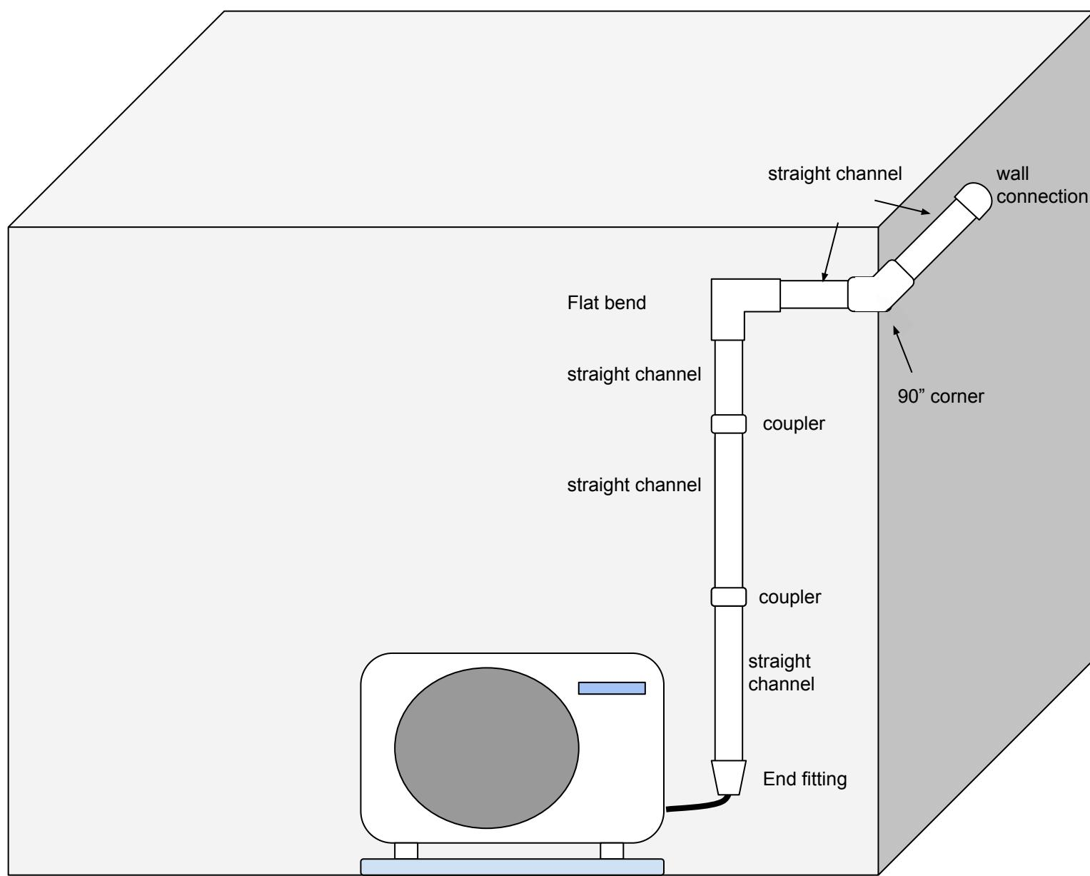
8-10 feet straight up the wall connecting into the soffit using 3 inch wide Diversitech covers:
