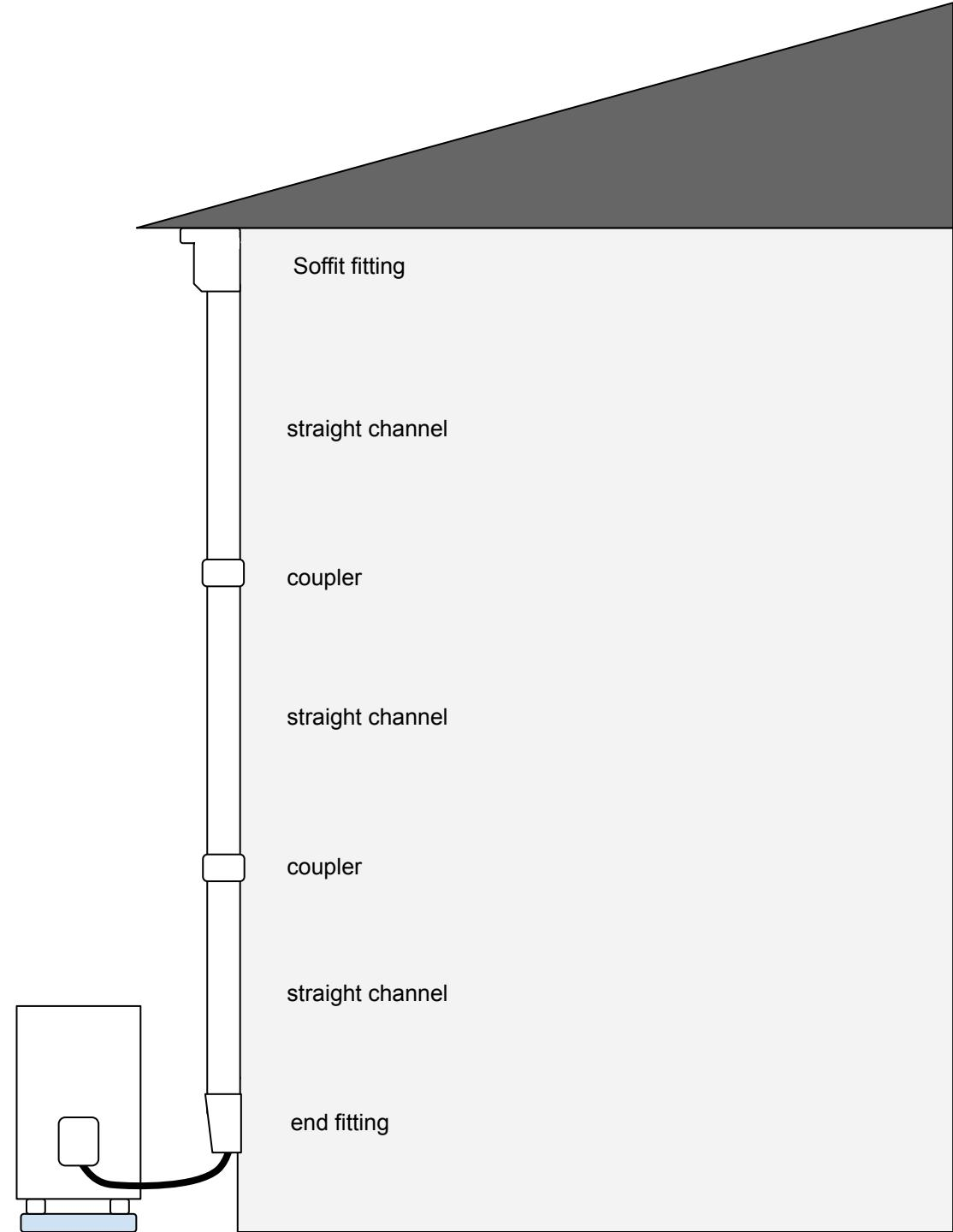
Starting with 4 inch Diversitech line set covers and reducing to 3 inch covers (on the horizontal section). Up 8 feet with two  $\frac{1}{4}$   $\frac{3}{8}$  diameter line sets, then take one line set continue up and enter the structure at 9 feet up. Take the other line set to the right for 10 feet, go up 1 foot vertically at the end of the line set run and enter the structure at 9 feet up:
