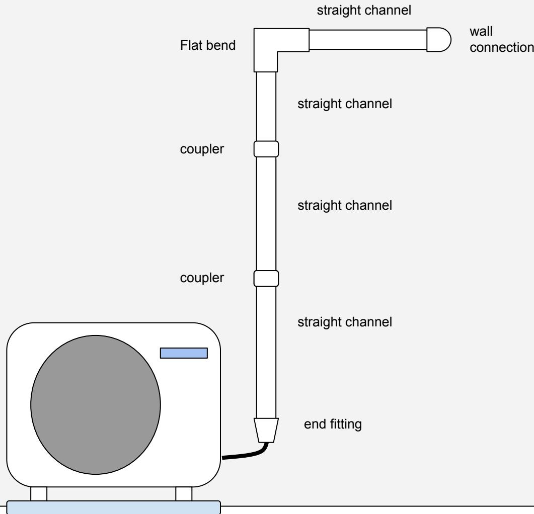
8 feet straight up the wall with a bump-out on the wall using 3 inch wide Diversitech covers:
