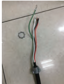
Remove the ring by turning counterclockwise
