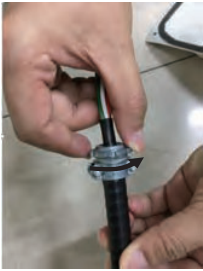
Remove the ring by turning counterclockwise
