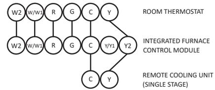
Thermostat - Two-Stage Heating with Single-Stage Cooling
