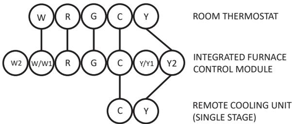
Thermostat - Single -Stage Heating with Single-Stage Cooling
