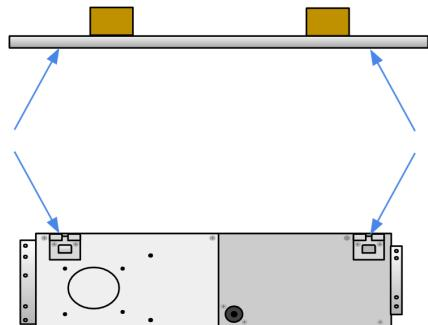
Select 3/8 inch threaded rods that match the last measurement x4 . This will allow for flexibility during the installation. It is common to cut the threaded rod to size using a hacksaw or sawzall.
