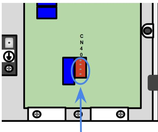
Red 4 pin connector from the wall controller to the red 4 pin CN40 port.
