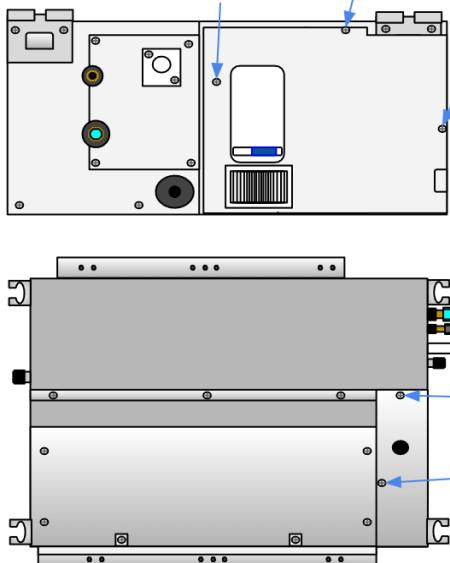
Remove the three screws on the side and the two screws on the bottom to expose the wiring connections.
