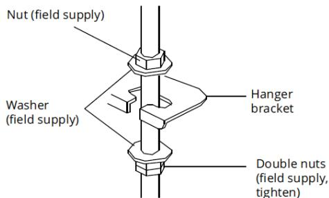
**Attach the hanger brackets to the threaded rods. Be sure to fix it securely by using a nut and washer from the upper and lower sides of the hanger bracket.**
