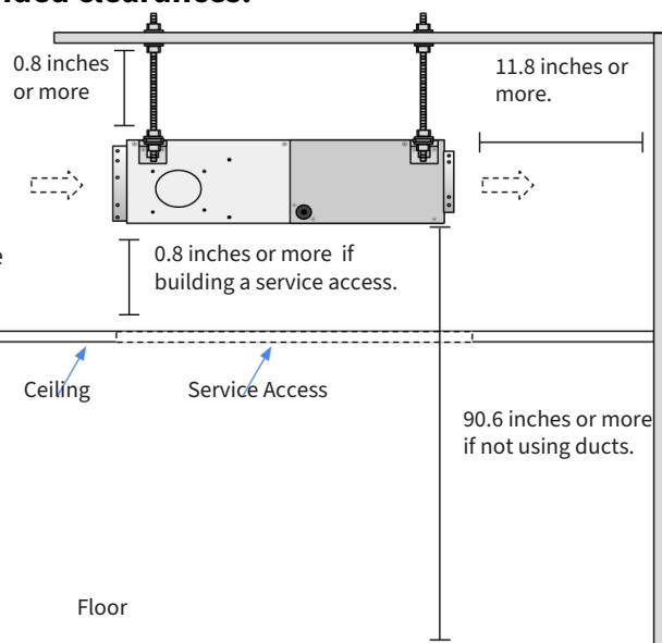
If suspending the indoor unit directly into the space with no ductwork, a minimum clearance from the floor to the bottom of the indoor unit is 90.6 inches or more.
