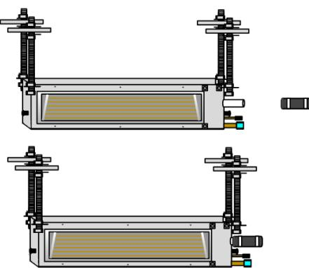
Seat the adapter as far on the drain connection as you can. Use the included metal clamp to secure the adapter
