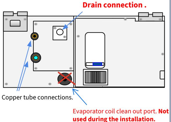
**Connect the the copper tubes to the indoor unit.**
