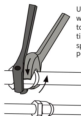
Use a standard wrench and a torque wrench to tighten to the specified foot pounds of torque.
