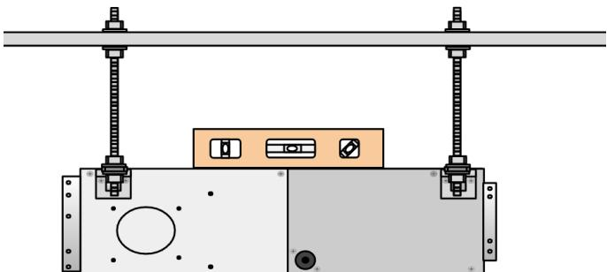
**Ensure that the unit is level. Failure to do so can cause operational issues and condensation leaks.**
