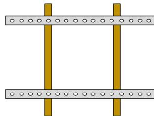
Above where the indoor unit will be installed, you need to use unistrut or 2x4 lumber to create a **solid, secure, level** structure for the threaded rod to install into. Hanging hardware does not come with the system.
