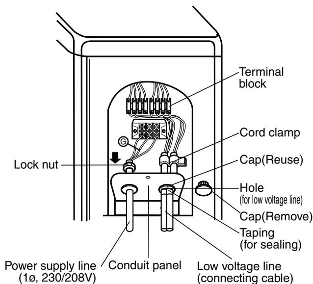
When connecting each power wire to the corresponding terminal, follow instructions "How to connect wiring to the terminals" and fasten the wire tightly using the screw on the terminal plate.
