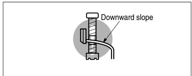
2. See below for examples of incorrect drain pipe applications, which will cause poor condensate flow.
