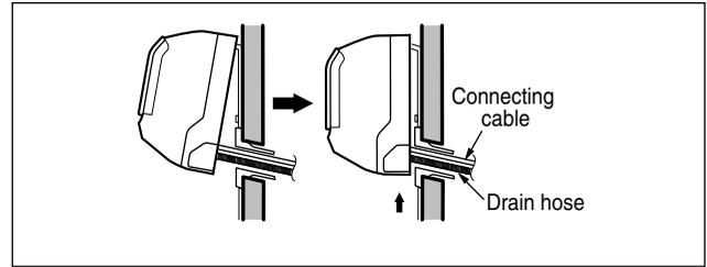
**Connecting the piping to the indoor unit and drain hose to drain pipe.**
