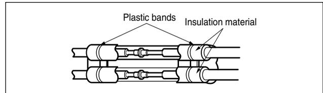
3. Bundle the piping and drain hose together by wrapping them with vinyl tape over the range within which they fit into the rear piping housing section.
