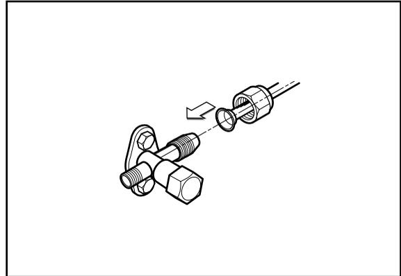
Finally, tighten the flare nut with torque wrench until the wrench clicks.
