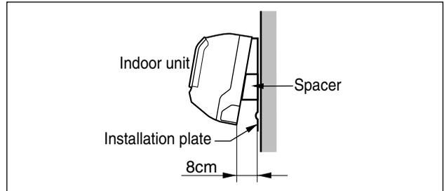
**Connecting the piping to the indoor unit and the drain hose to drain pipe.**
