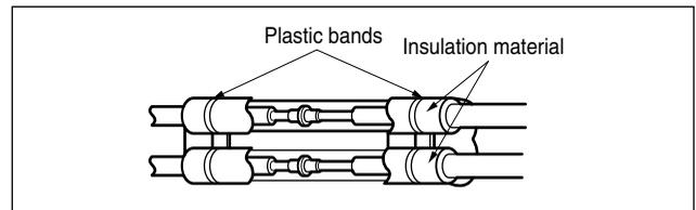
3. Bundle the piping and drain hose together by wrapping them with vinyl tape, enough to cover where they fit into the rear piping housing section.
