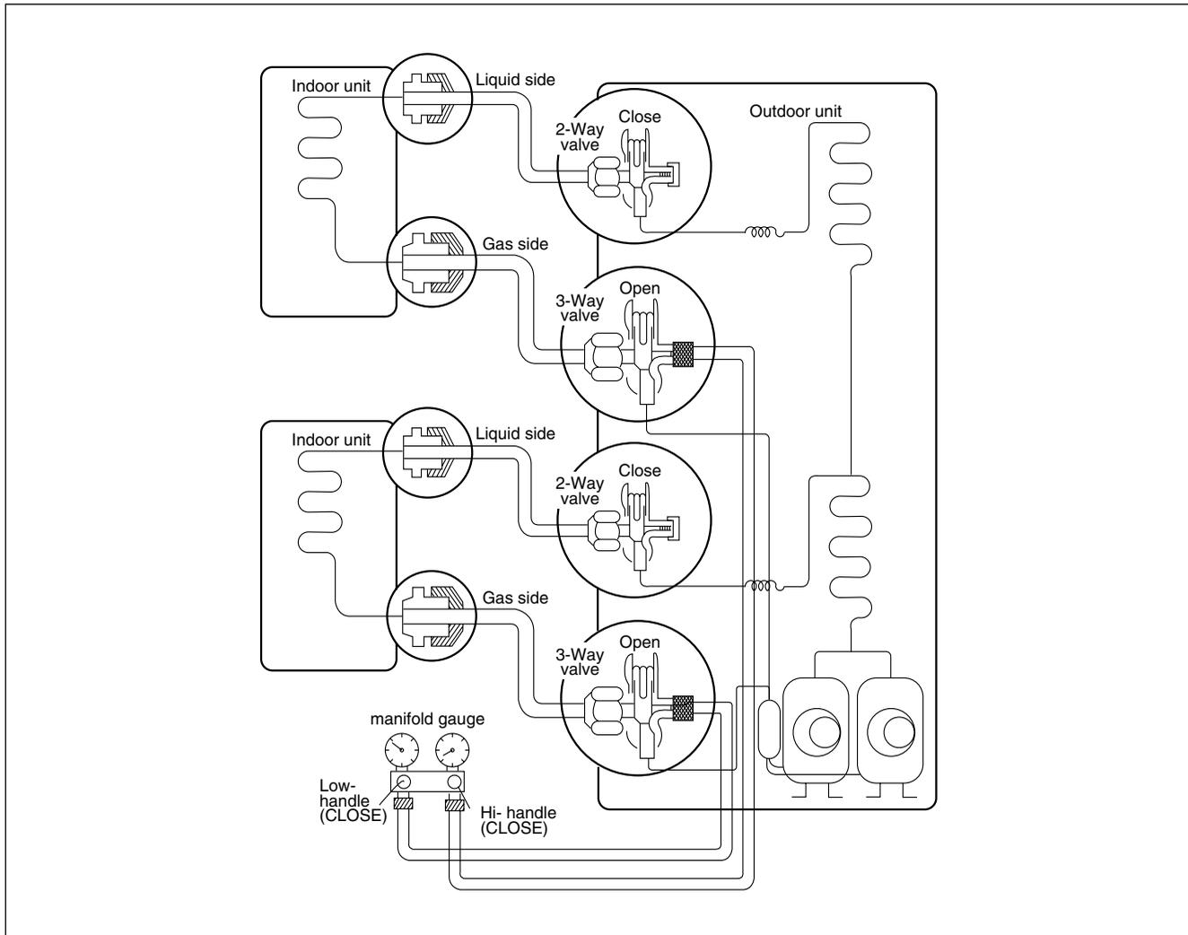
**• Procedure****1. Confirm that both the gas side and liquid side valves are set to the open position.**
