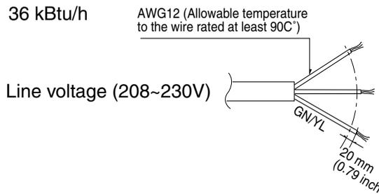
The power connecting cable connected to the indoor and outdoor unit should comply with the following specifications: ETL recognized and CSA certified.
