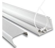
DiversiTech recommends attaching the base to the wall or ceiling and the line sets to the system every 15" to allow for the system to carry the full weight of the line sets.
