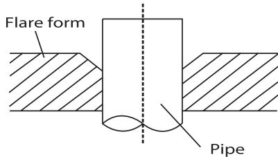
6. Place flaring tool onto the form.
