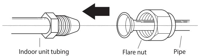
3. Tighten the flare nut as tightly as possible by hand.
