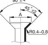
8. Remove the flaring tool and flare form, then inspect the end of the pipe for cracks and even flaring.
