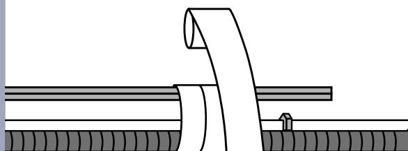
Use PVC electrical tape to secure every 3-4 feet, then install zip ties over taped sections.
