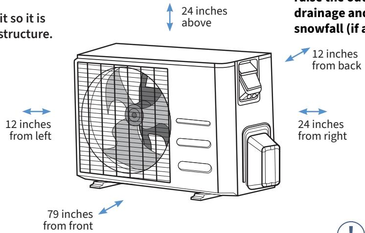
If used for heating, it is recommended to raise the outdoor unit to allow for proper drainage and keep it clear of expected snowfall (if applicable).
