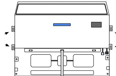
Secure the unit to wall studs with lag screws. If attaching to another wall type, use the appropriate mounting fasteners. Mounting fasteners, not included.
