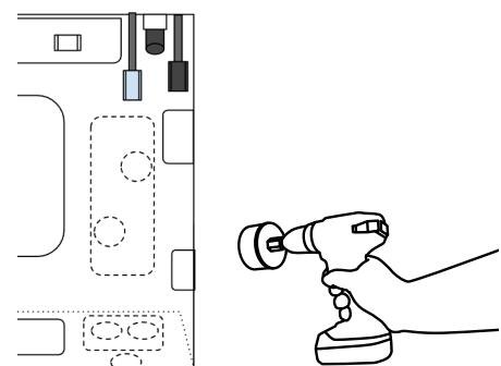
There are knockouts on the lower, rear, right side, and the bottom of the indoor unit. Using the bottom knockout is recommended for most installations.
