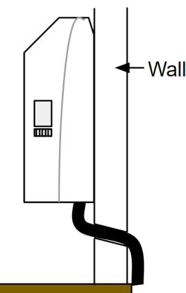
Run the drain to the ground, at least 12 inches from the structure.
