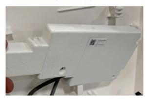
Secure the panel back into place with the same phillips head screw.
