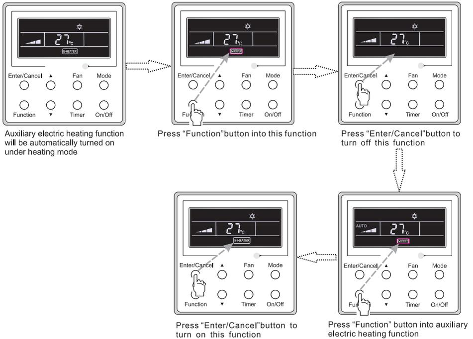
Fig.14 E-heater Setting
