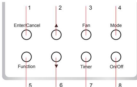
Fig. 3 Buttons on the Wired Remote Controller
